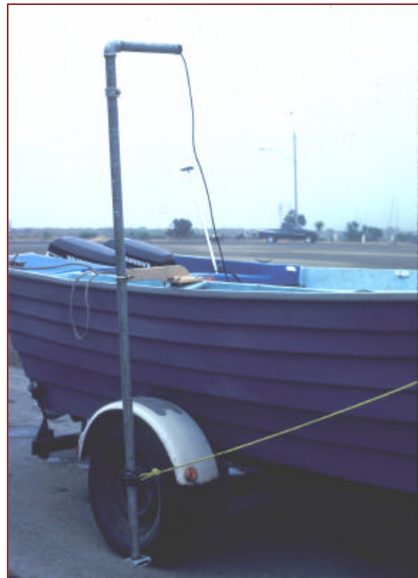
Figure 5. Boat Rigged for Mobile Tracking with Directional Hydrophone
